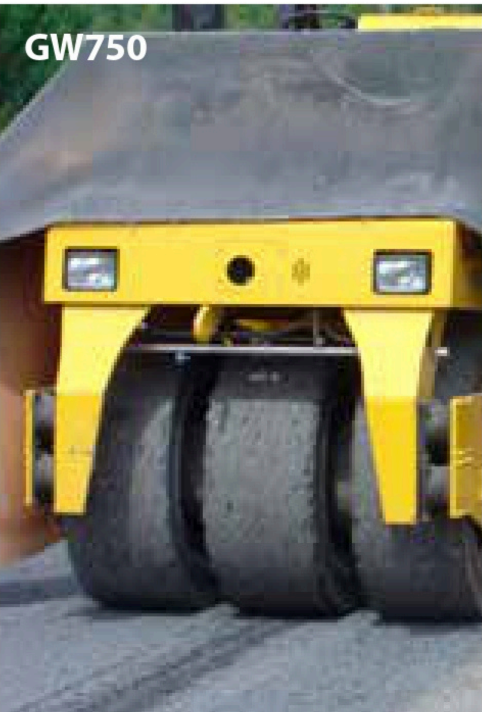
Fig 2. Chip seal pavement finished by GW750
