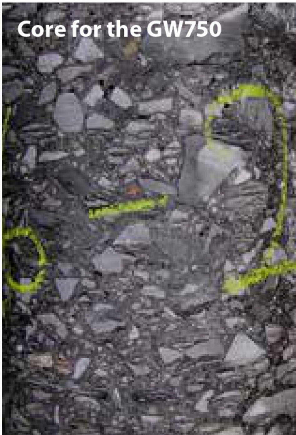
Fig 5. Uniform compaction throughout thick lift ( 27 cm with 3.8cm aggregate size ) HMA pavement layer by two different rollers
