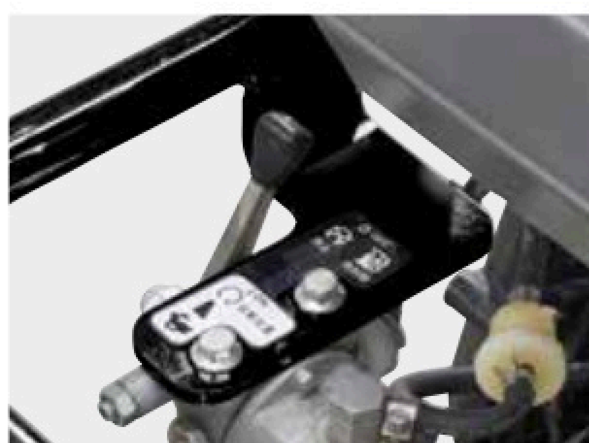
One throttle lever (Engine-off, Fuel-off, Throttle adjustment)
