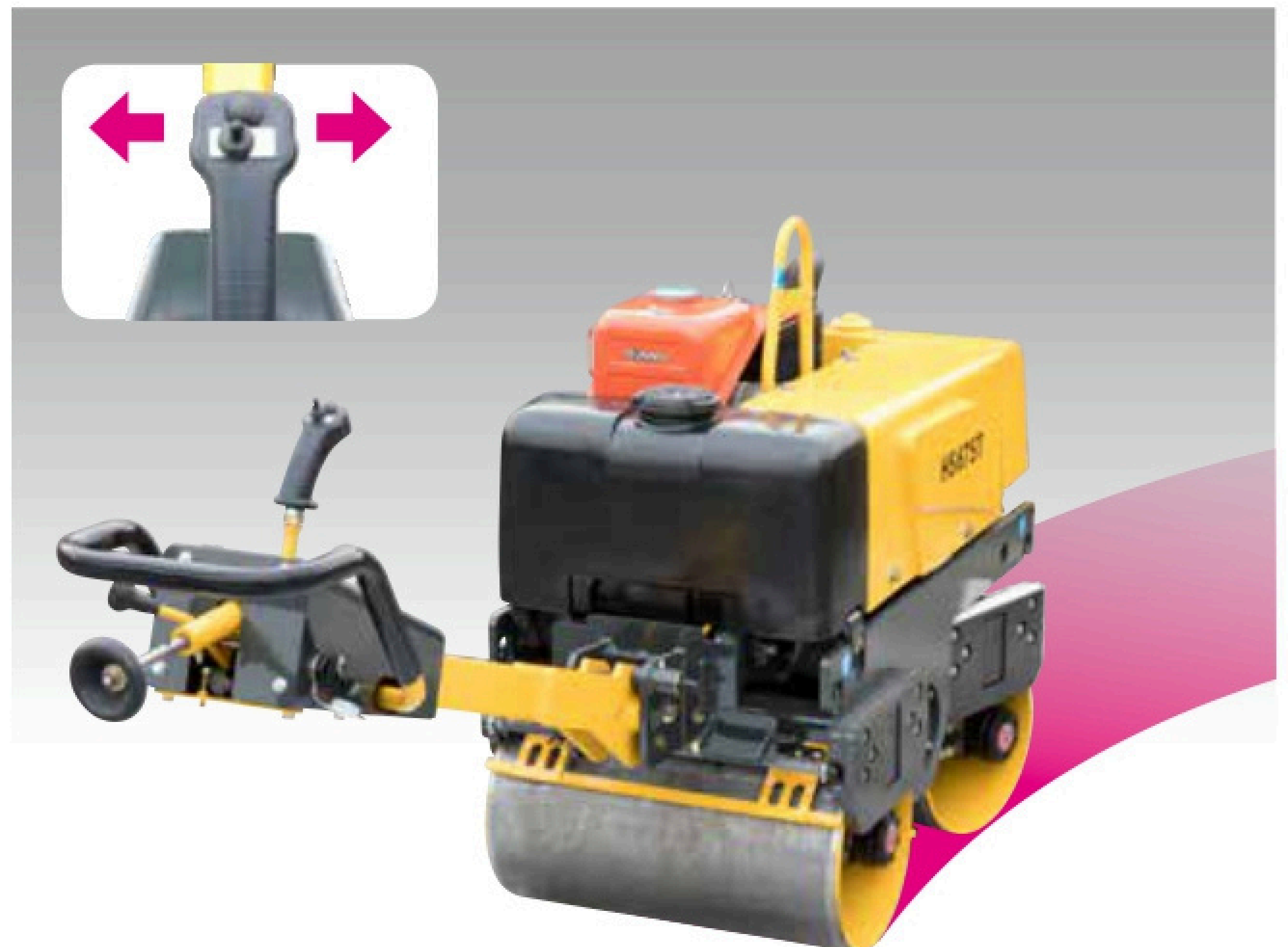
Power steering (HS67ST) Steering angle: +/- 15 degrees
